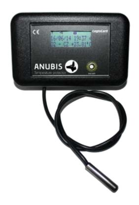
**ANUBIS** GSM thermometer allows temperature logging and in case of overtemperature alerting over SMS or e-mail. **ANUBIS** temperature logger stores temperature values in its memory and it regularly sends data over GPRS to our server. Reports and actual status is accessible 24 hours a day on our website. Current temperature can be also seen on the built-in display. Firmware upgrade is fully automatic (done on background and without interrupted operation).
